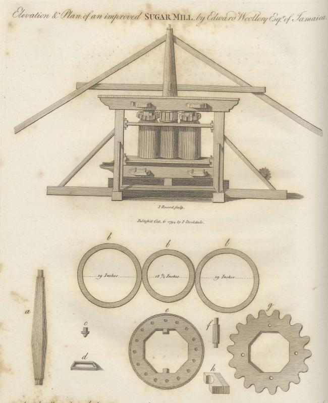
a. the side roller gudgeon. I the rollers or cylinders. C. pivot to each roller, called the capoose . d the step on which the capoose turns. C the lantern wheel of the trundle or wallower of which there are sixteen in the lantern wheel of correspondences of which the rollers. A the side brack to the rollers.
